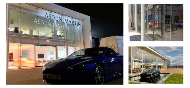
This Aston Martin showroom at Atmell Way, Silver Link in Newcastle shows how impressive sliding doors can look. The installation at this showroom comprised the **record STA 20 DUO** double doors with radar activation and presence sensor for two way traffic. The construction also included battery back-up in case of power failure or fire alarm activation.
