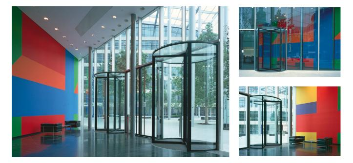
The east entrance at Tower Place in london was designed by architects Foster and Partners. This installtion is a fully automatic **record K41** four wing revolving door and has an all-glass drum with visible parts anodised. The operating drive for this revolving door is concealed beneath the floor in a casing which protects it from water and dirt.
