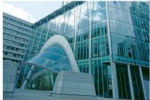
The entrance to serviced offices at City Point in London. A **record K41** 4 wing revolving door has been installed here with the underfloor drive unit connected by a continuous drive shaft. The drum wall consist of glass and all visible components with a brushed stainless steel finish.
